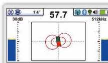
Sonde Screen - arrow guidance showing direction to the sonde and depth of cover
